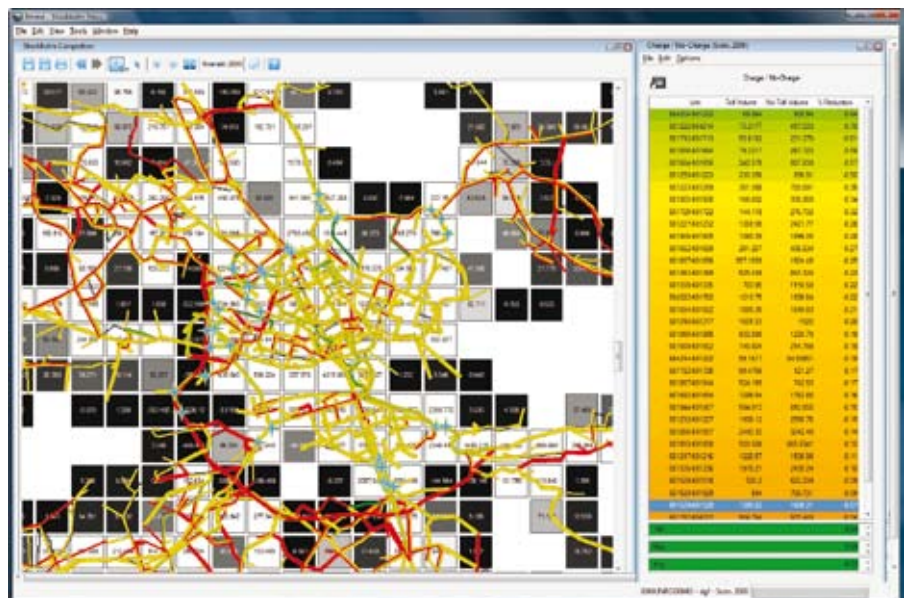
Routes, volumes, and travels times for trips can be determined using Emme forecasting software
